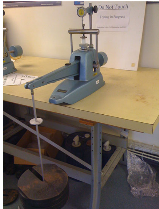
Fig. 14 Apparatus used to measure creep
